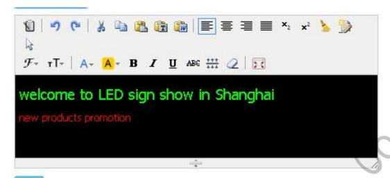
Hint Press Enter to separate next page, Press Shift + Enter to new a line. Define the following string instead of the value of sensors in terminal: %c is celcius, %f is fahrenhite, %h is humidity, (%c1 %f1) or (%c2 %f2) round to 1 or 2 digit(s) after the decimal point
